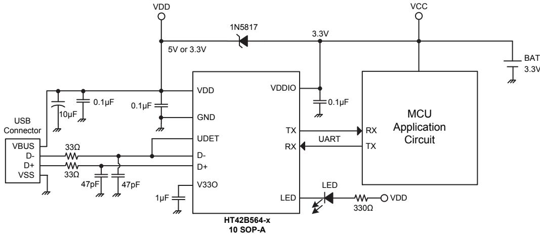
Note: 1. The V<sub>CC</sub> voltage must be less than the V<sub>DD</sub> voltage. The V<sub>CC</sub> supply can be sourced from a Li-battery.
